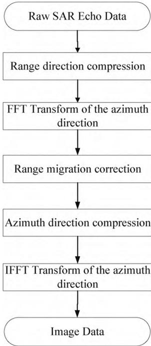
Figure 4 Block diagram of RD algorithm
