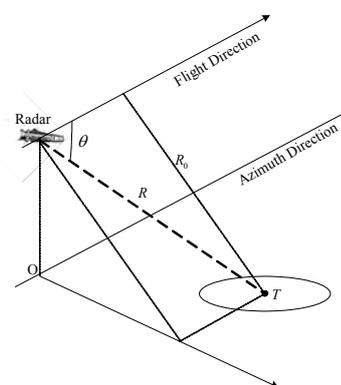
Figure 1. Geometry relation between radar and target
