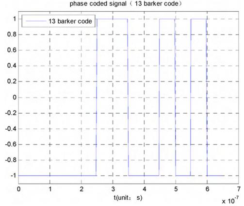
Figure2 Waveform of the baker code
