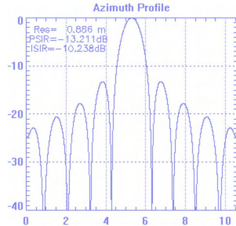
Figure 6 Compression result after azimuth direction
