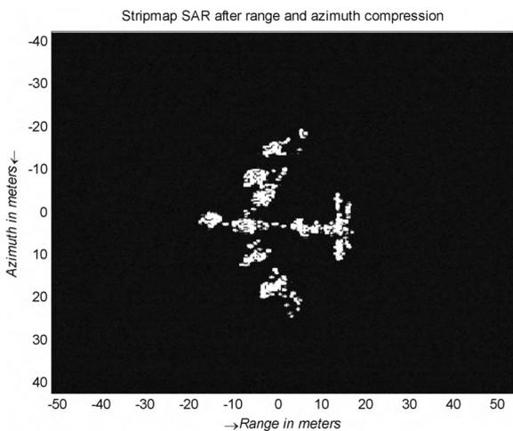
Figure 9 Image result of the aeroplane
